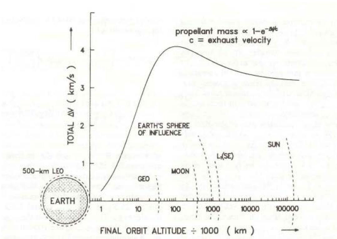
Fig. 3. Delta-v vs circular orbit altitude above the Earth.
