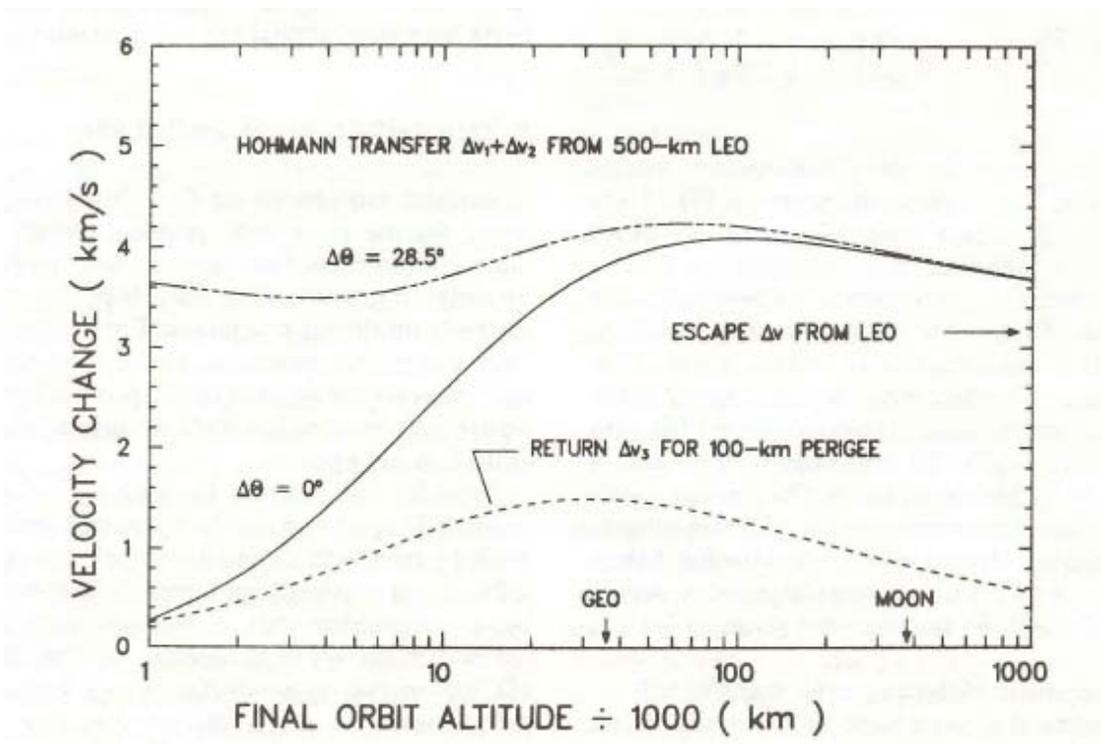
Fig. 4. Earth orbital transfer missions.
